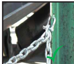
The other end of chain anchored with a 6mm D Shackle, which is adjustable.
