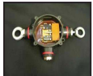
Switch connections inside Rip Detector. Pin is held in position with two spring loaded ball bearings.
